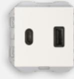
20000296 | -090 -091 -093 -094 -095 -096 -097 -098 | Cargador USB doble A+C 3,1A Quickcharge
